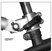
Pictured above left is the quick release lever in the closed position. Above right is the quick release in the open position. IMPORTANT: DO NOT TIGHTEN THE QUICK RELEASE LEVER AS THOUGH IT WERE A WING NUT. Tighten and then press the lever firmly into closed position.
