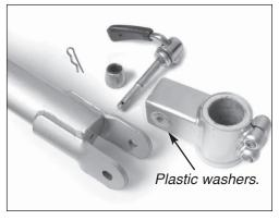
Pictured top is the hitch assembly disassembled. Below left is the seatpost with part of the hitch assembly attached. Pictured right is the nut and bolt of the quick release opposite the lever. PIN MUST BE FULLY ENGAGED.
