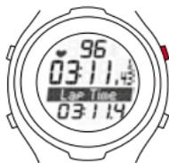
5. To finish training, simply press the START/STOP button. The stopwatch stops. To reset the values to zero, press and hold the START/STOP button. To exit the training mode, press and hold the TOGGLE (-) button.
