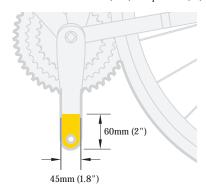
2 FlashStand FAT is designed to be used on bikes with crankarm distance from the ground between 80mm and 180mm (3.2"~7").
