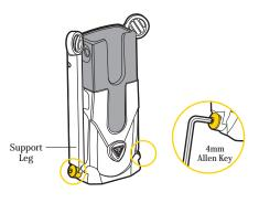
Adjust FlashStand FAT height to make sure your bike is within the recommended angle of 83°~86° (from horizontal plane) for stability of your bike. Improper installation or lean angle may cause your bike to fall and cause damage to it and/or FlashStand FAT.
