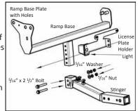
the holder with the screws provided with the light. Make sure the light is facing towards the license plate.
