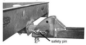
Insert the spring pull pins into the two holes on the ramp when you stand the ramp upright. See the figure.
