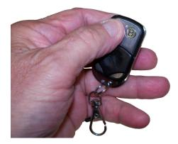
3. Remove the battery and continue to press the "A" button on the remote.
