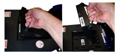
4. Continue to press the "A" button on the remote and install the battery. Continue to press the "A" button for 2 seconds after the battery is installed. Release the "A" button and now the remote is paired with the Zoome Auto-Flex.
