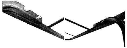
18. Slide the canopy over the main frame with the larger flap in the rear.
