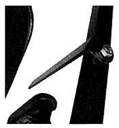
9. Locate and remove the nut from the armrest pivot bolt.
