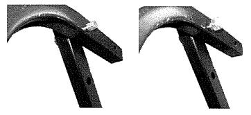
17. Pivot the main frame upward to align the forward holes on each side with the forward holes in the "L" bracket. Slide a bolt through these holes. The head of the bolt is on the outside of the frame. Place a nut on each of these bolts and tighten all four nuts and bolts on the main frame.
