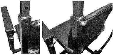
16. Position the main frame so that the rear holes align with the rear holes in the "L" bracket. Slide a bolt through these holes. The head of the bolt is on the outside of the frame. Tighten by hand a nut onto each bolt.
