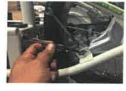
6) With two (2) 8 mm wrenches, remove the cable guide bracket from the frame and brake plate. Keep all the herdware together.
