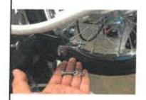
7) With two (2) 15 mm wrenches, loosen the axie nuts from the wheel. Slide the wheel forward, remove the chain from the sprocket and remove the wheel. Note the sequence of the hardware.
