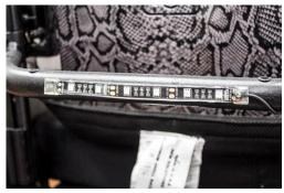
Lights are connectable to each other with an easy snap. Run wires along chair and secure as you see fit. Attach battery cables to battery with supplied terminal connectors.
